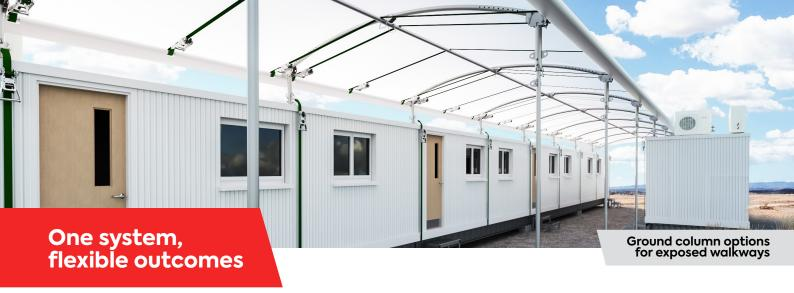
RhinoSite's temporary walkway shelter system is available in 3 meter modules for a perfect fit across all standard 6m & 12m portable buildings. Modules can be easily joined to cater for any length of walkway, varied building sizes and exposed walkways. The strong, galvanized steel frame is positioned and secured with wire lock pins before tensioning using a unique heavy duty fabric cover and nylon ratchet straps to achieve a robust solution.
